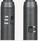
(1) Adjust the three position level control according your needs (0dB, +10dB,+20dB)
